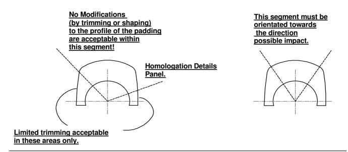
**Note:** <u>DO NOT</u> apply the adhesive to the padding before trial fitting is completed. It is important that the Homologation details panel is not compromised (at least one complete panel should remain) and is installed to be visible to and enable checking by the Scrutineer.
